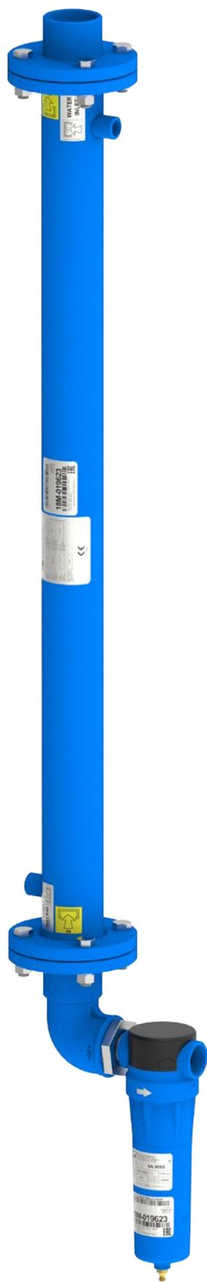
The water after-coolers are composed of two parts: a high efficiency shell in tube air-water heat exchanger, offering little pressure drops to cool air, and a cyclone condenser separator to separate and eliminate the condensed water.
